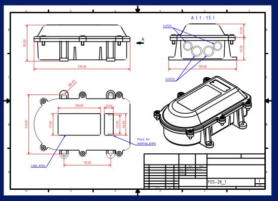
Space for two troughgoing cables up to 7 mm
