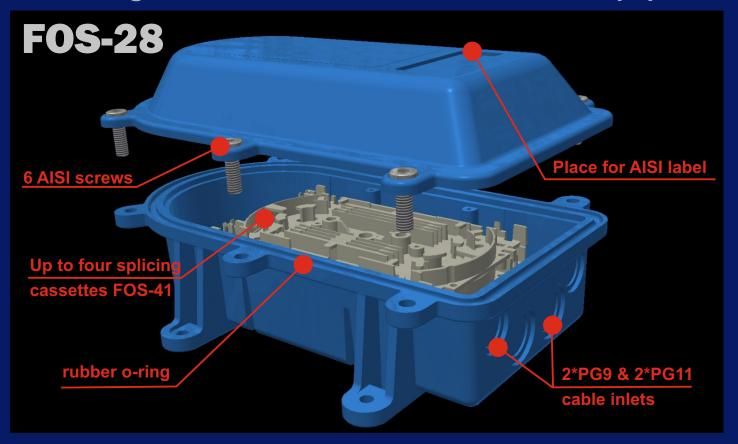
FOS-28 is outdoor fiber optic enclosure for FTTH applications. There can be installed up to four splicing cassettes, up to 48 splices. Optional adaptor plate and pole fixings available
