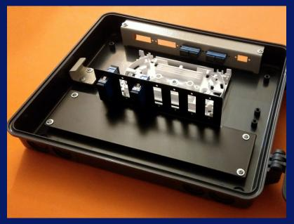
If using FOS-54 as fiber-optic enclosure, You can install here splicing cassette FOS-41, backplate with various fiber optic adapters and internal switching panel. Also, here is options with two types of fixings for splitters.
