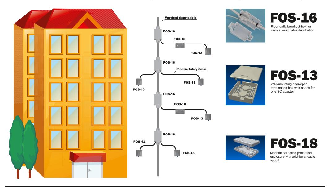
Riser cable installation in apartment house using fusion splicing
