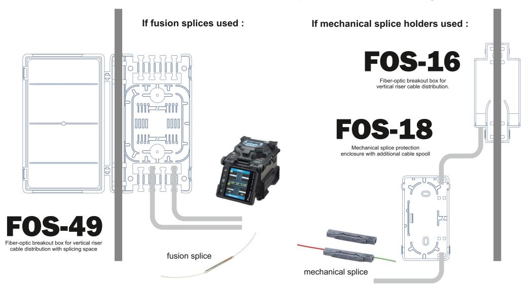
Vertical riser cable installation in apartment house using mechanical splices
