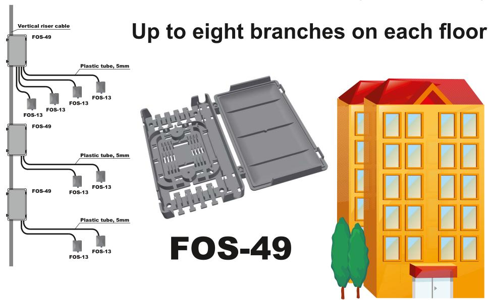
Riser cable installation in apartment house using distribution box FOS-49
